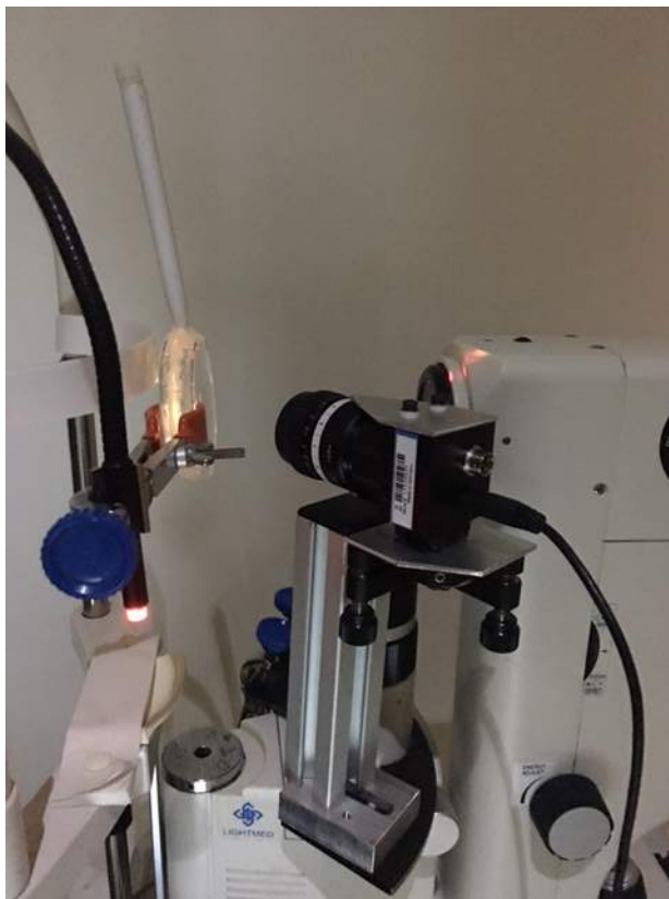
Figure 3.1.2.4 A photo of how imaging system works after arc was attached to the laser system.
