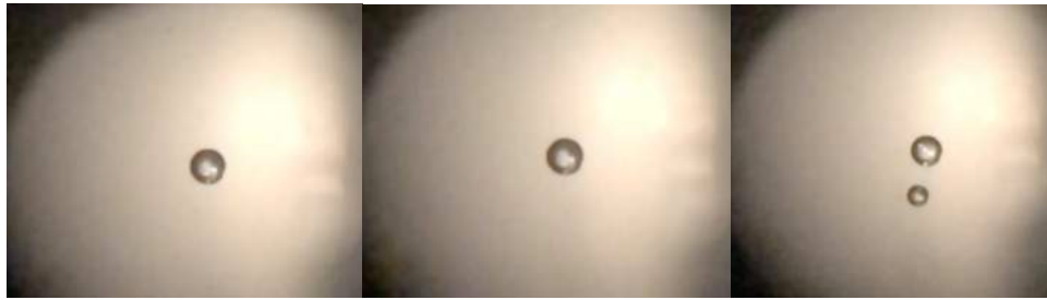
Figure 4.1.2 Bubbles that are created with different laser energy levels are showed. Bubble in the left image created with 1mJ laser energy. Bubble in the middle image created with 1.2 mJ laser energy and bubbles in the right image created with 1.5 mJ. It can be seen that couple of bubbles appeared when laser energy increased.
