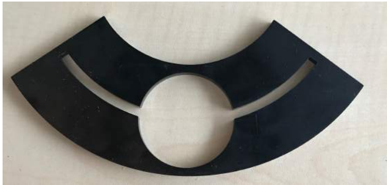
Figure 3.1.2.3 Arc is created with a CNC system.
