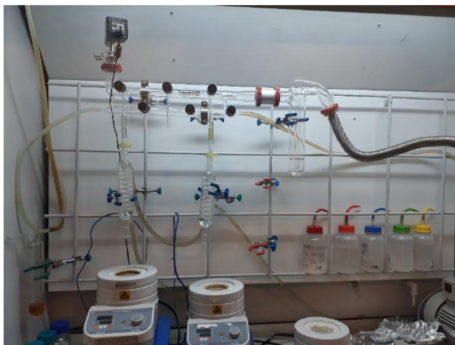
Figure. 3.8.4 The colloidal nanocrystals synthesis system in a fume hood
