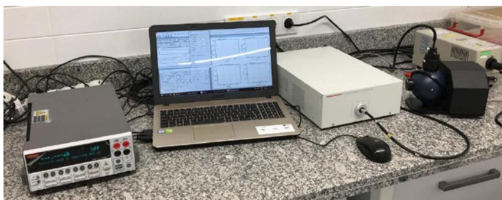
Figure. 3.8.2 The external quantum efficiency measurement system C9920-12 for light emitting diodes. From left to right: Keithley 2400, PC with dedicated software, PMA-12, integrating sphere and halogen light source.
